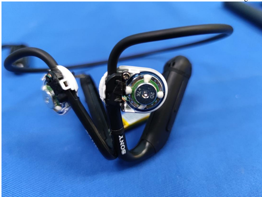
Figure 2 Inside Configuration of the EUT
