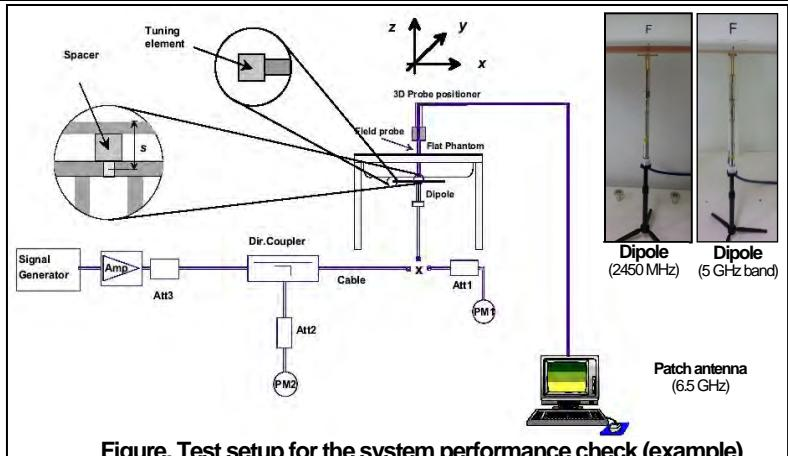
**Figure. Test setup for the system performance check (example)**
