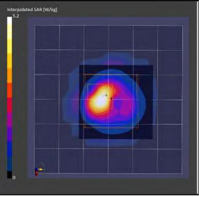
Remarks: \*. Date tested: 2023-01-24 ;Tested by: Hiroshi Naka; Tested place: No.7 shielded room; Ambient: (22-23) deg. C. / (50-75) %RH; Liquid depth: 150 mm;
