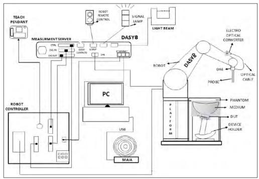
The DASY8 system for performing compliance tests consist of the following items:
