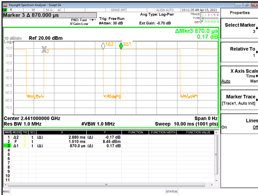
Equation 8-1 Bluetooth Duty Cycle Calculation for Right ear
