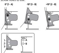
3 At the desired angle, tighten the 2 screws through the screw holes (upper or lower) that match the display angle.
