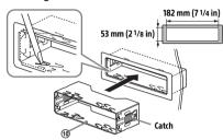
2 Mount the unit onto the mounting sleeve (1) then attach the trim ring (2).
