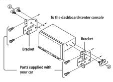
When mounting this unit to the preinstalled brackets of your car, use the mounting screws ② in the appropriate screw holes based on your car: T for TOYOTA and N for NISSAN.
