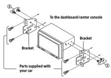
When mounting this unit to the preinstalled brackets of your car, use the mounting screws ② in the appropriate screw holes based on your car: T for TOYOTA and N for NISSAN.
