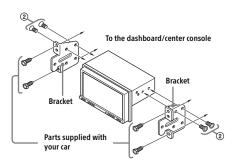
When mounting this unit to the preinstalled brackets of your car, use the supplied screws ② in the appropriate screw holes based on your car: T for TOYOTA and N for NISSAN.
