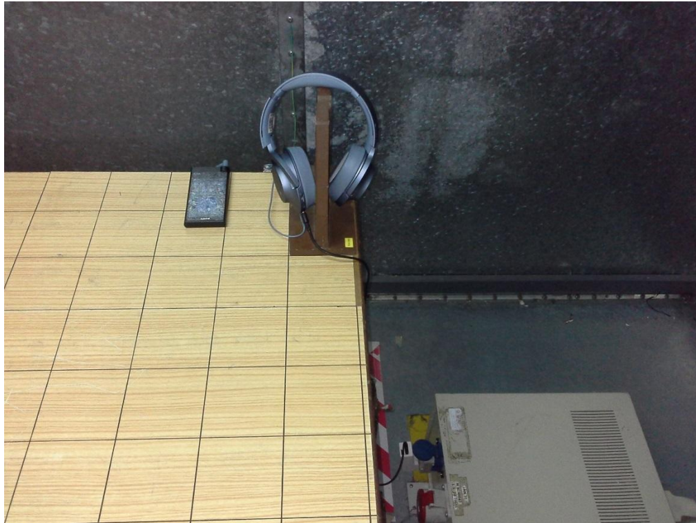
Conducted Emissions Test Setup (Front View)
