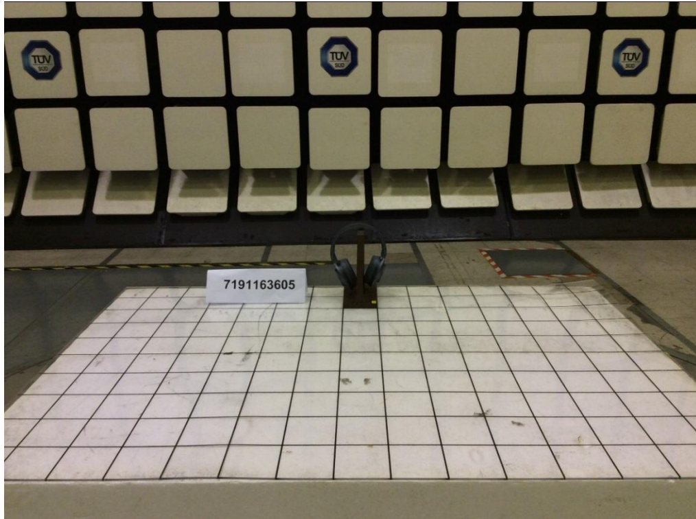
Radiated Emissions Test Setup (Front View)
