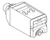
3 Insert two new AA batteries into the battery compartment with ⊕ and ⊖ polarities in the correct orientation.
