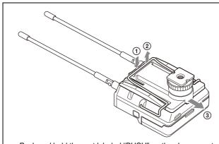
Push and hold the part labeled "PUSH" on the shoe mount adapter (①), and disengage the horizontal part of the belt clip from the horizontal groove on the shoe mount adapter (②). Then, push the shoe mount adapter in the direction of the arrow (③).
