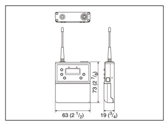
$63 \times 73 \times 19 \text{ mm } (2^{1}/_{2} \times 2^{7}/_{8} \times {}^{3}/_{4} \text{ in.})$ (width / height / depth) (excluding antenna)
