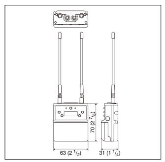
$63 \times 70 \times 31 \text{ mm } (2^{1}/_{2} \times 2^{7}/_{8} \times 1^{1}/_{4} \text{ in.})$  (width / height / depth) (excluding antenna)
