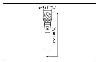
$\emptyset 48 \times 258 \text{ mm } (1^{15}/_{16} \times 10^{1}/_{4} \text{ in.})$ (diameter / length)
