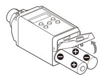
4 Close the battery compartment cover and turn the knob clockwise to lock the cover.
