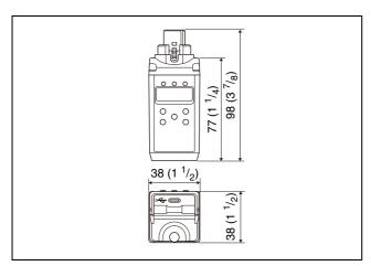
$38 \times 98 \times 38 \text{ mm} (1^{1}/_{2} \times 3^{7}/_{8} \times 1^{1}/_{2} \text{ in.})$ (width / height / depth)
