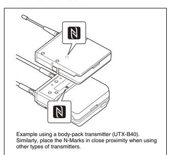
Information about the channel set on the tuner is sent to the transmitter, and then the transmit channel is set. "COMPLETE" is shown on the display of the transmitter and tuner, and the transmitter vibrates when setup is finished.
