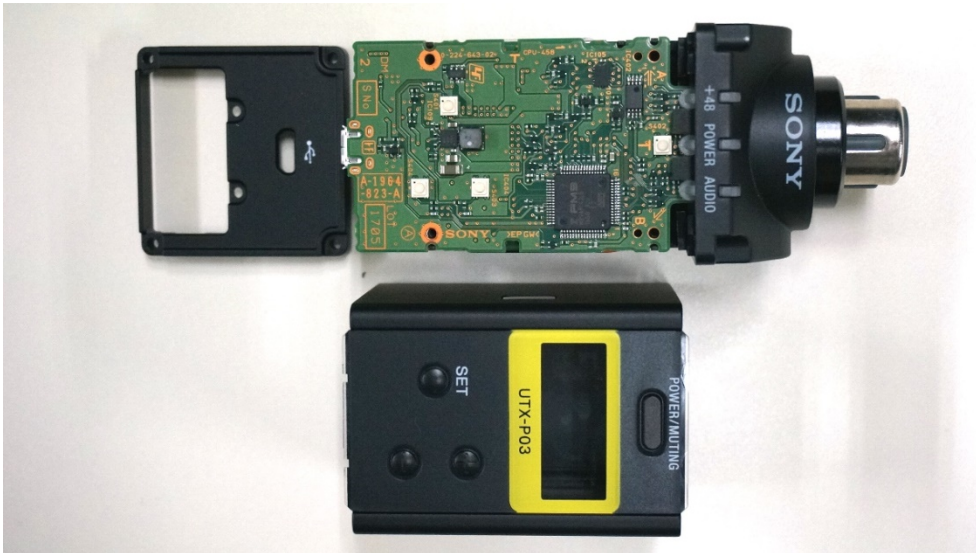
Fig.1: Removed the Case (Place of board CPU-458)
