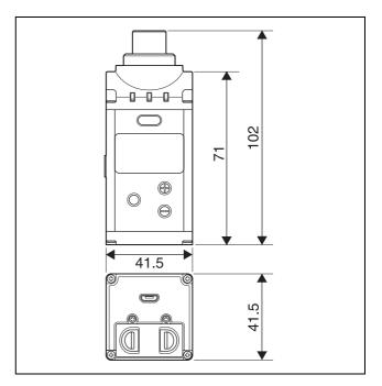
$41.5 \times 102 \times 41.5 \text{ mm}$  $(1^{11}/_{16} \times 4^{1}/_{8} \times 1^{11}/_{16} \text{ in.})$ (width / height / depth) (including the audio input connector) Mass Approx. 145 g (5.1 oz) (excluding batteries)
