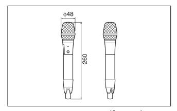
$\phi$  48 × 260 mm (1 <sup>15</sup>/<sub>16</sub> × 10 <sup>1</sup>/<sub>4</sub> in.) (Diameter / length) Approx. 260 g (9.2 oz) (excluding batteries)
