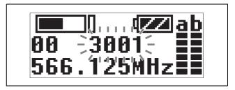
**4** Use the + or – button to select the desired channel number, then press the SET button.
