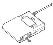
3 Insert two new AA batteries into the battery compartment with ⊕ and ⊖ polarities in the correct orientation, and close the the compartment.
