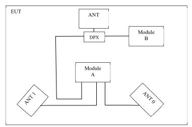
The EUT has module A and module B.
