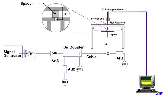
Fig 7.1 System Setup for System Evaluation
