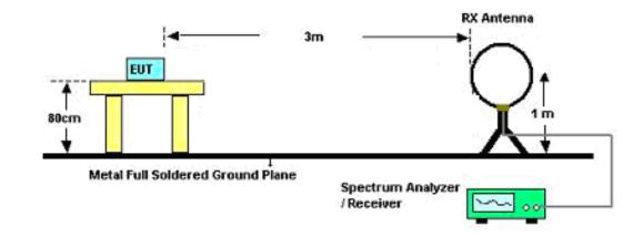
For Radiated Emissions: 30MHz~1GHz
