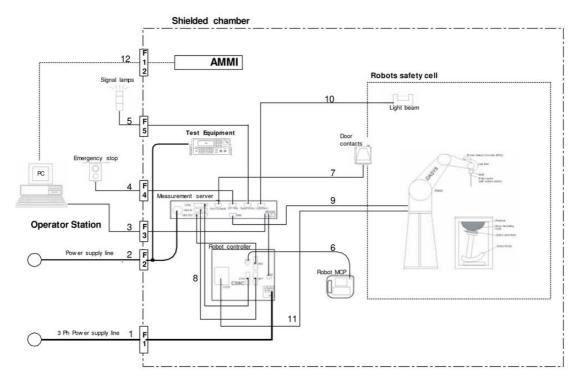
The DASY5 system for performing compliance tests consist of the following items:
