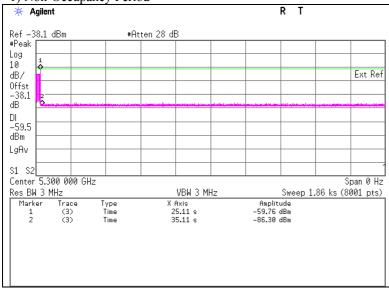
Marker 1 : End of Burst : 25.11 sec Marker 2 : End of Burst +10sec : 35.11 sec
