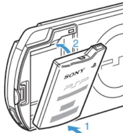
Align the tabs of the battery cover with the system and snap it in place.
