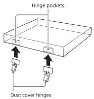
2 Align the attached hinges with the hinge pockets on the rear of your turntable and push in the dust cover.
