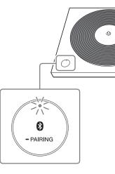
**3** Turn on the pairing mode for the playback device that supports BLUETOOTH wireless technology, to which you want to connect.
