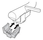
**3** Hold the cartridge body (1) with one hand, grasp the stylus with the other, and then pull the stylus in the direction of the arrow to remove it from the cartridge body.
