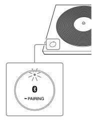
**3** Turn on the pairing mode for the playback device that supports BLUETOOTH wireless technology, to which you want to connect.
