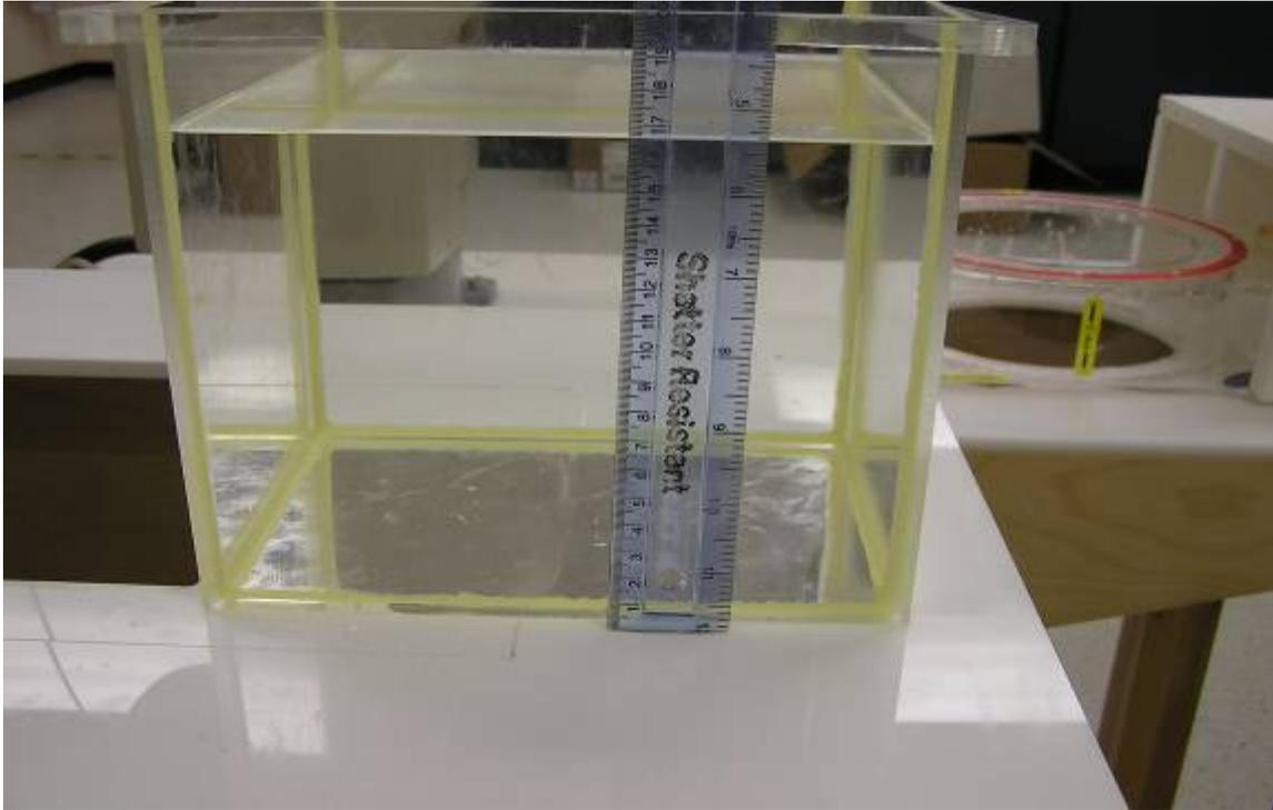
**Photo 2. Photo to demonstrate 15 cm Z-axis flat phantom**
