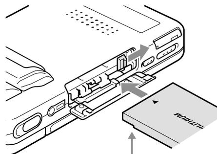
Face the battery terminal towards the display panel side
