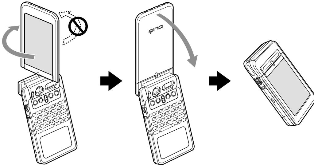
Open the display and rotate it as indicated by an arrow until it clicks into place
