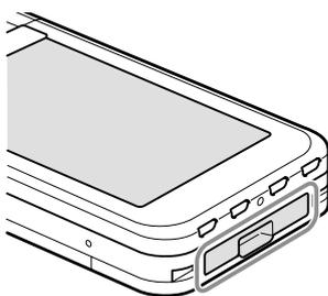
You can connect to the Internet by using the compact flash type data network card (from this point, referred to as network card).
