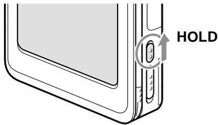
Protects your CLIÉ handheld from accidental tapping on the screen or pressure on the POWER switch when you are carrying your CLIÉ handheld. If you slide this switch while the power is on, the screen display turns off, even during an operation.
