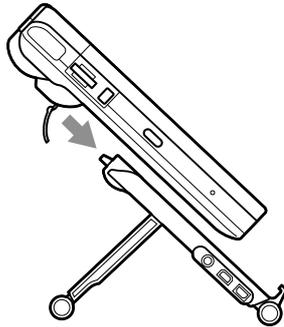
It takes about four hours for your CLIÉ handheld to be fully charged for the first time. The POWER LED indicator of your CLIÉ handheld turns off when charging is completed.
