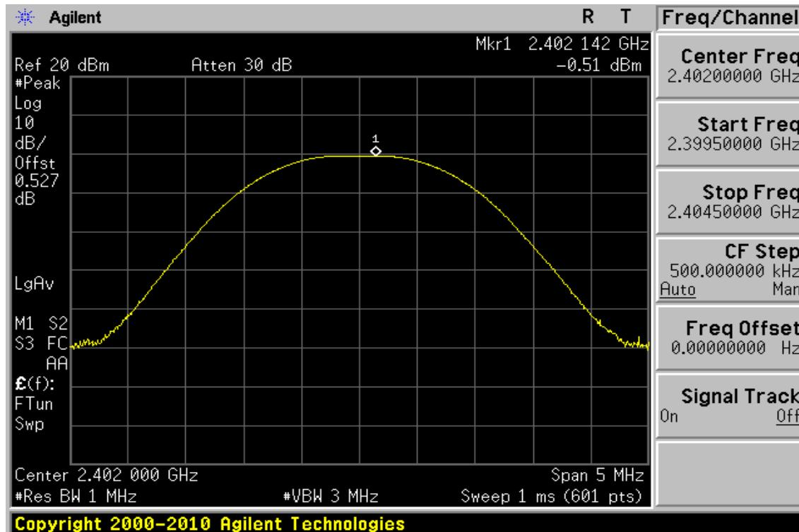
**Peak Power Output Data Plot (CH Mid) (BDR mode) GFSK**
