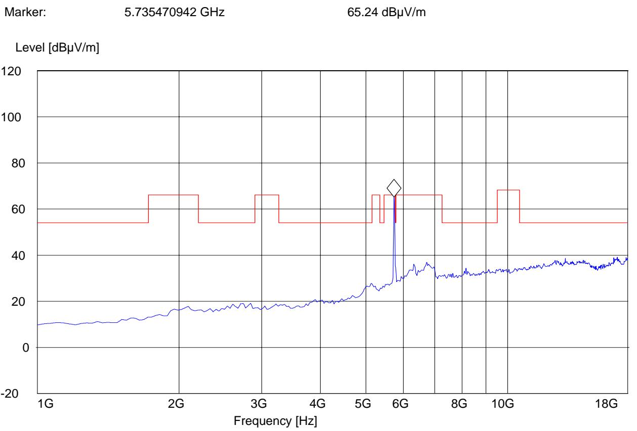
**1-18GHz (5785MHz)****Note: The peaks above the limit line is the carrier freq.****Note: Peak Reading vs. Average limit****CETECOM Inc., 411 Dixon Landing Road, Milpitas CA 95035, USA*****SWEET TABLE: "FCC 15.407 1-18G"***
