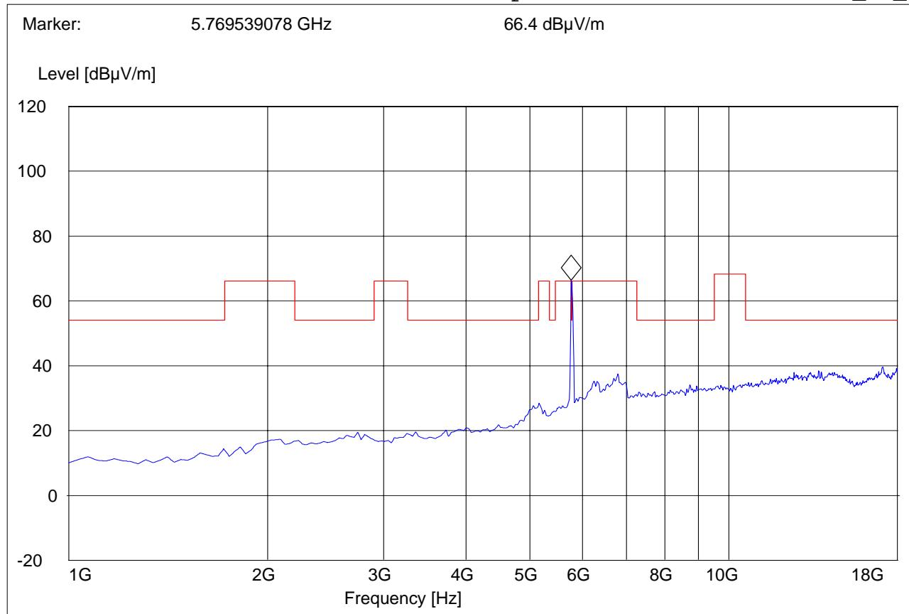
**1-18GHz (5825MHz)****Note: The peaks above the limit line is the carrier freq.****Note: Peak Reading vs. Average limit****CETECOM Inc., 411 Dixon Landing Road, Milpitas CA 95035, USA*****SWEEP TABLE: "FCC 15.407 1-18G"***
