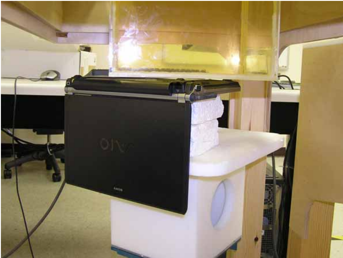
Photo 2: CDMA lap position antenna horizontal
