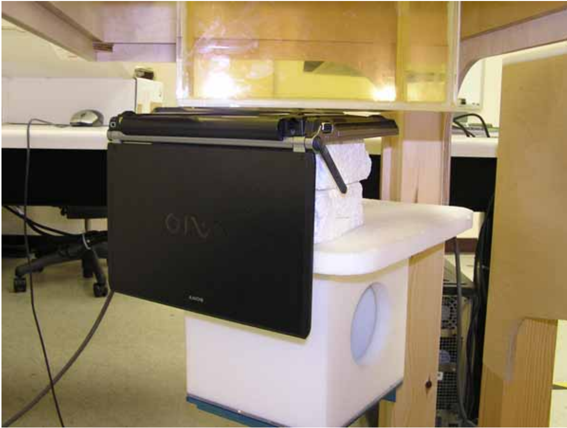
Photo 3: CDMA lap position antenna 45 degrees
