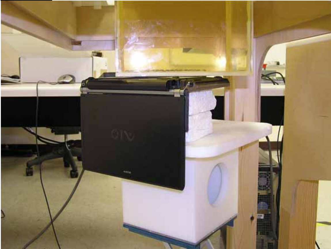
Photo 1: CDMA lap position antenna vertical
