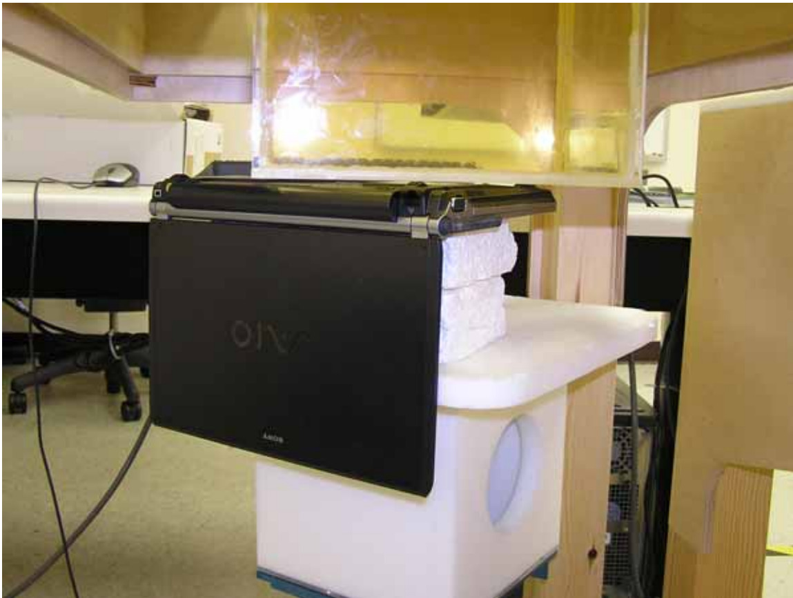
Photo 2: CDMA lap position antenna horizontal
