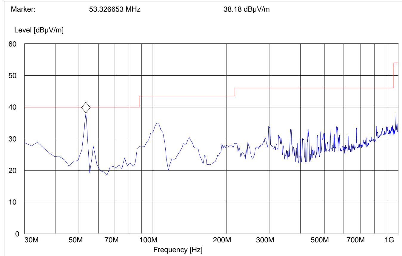
**EMISSION LIMITATIONS - Radiated (Transmitter)****§ 15.247 (d)****30MHz – 1GHz****Antenna: horizontal****This plot is valid for Collocation of both GSM & BT and WLAN & BT combinations.****(Worst-case plot)**
