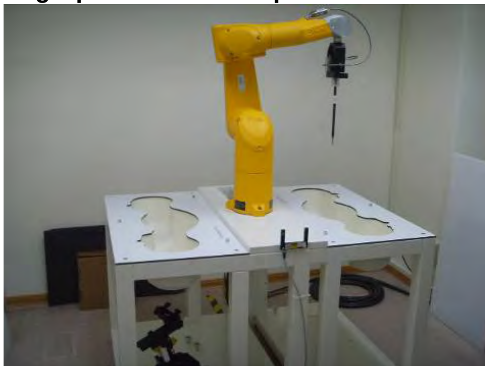
Fig.1 Photograph of the SAR measurement System
