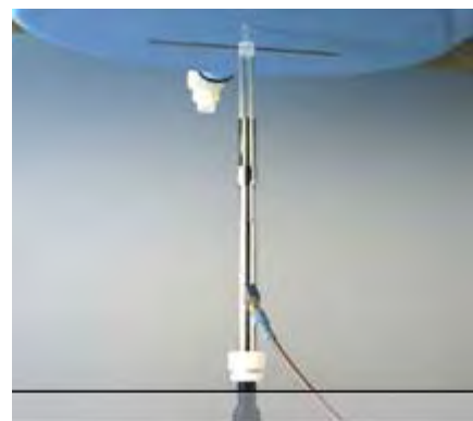
Photograph of the dipole Antenna
