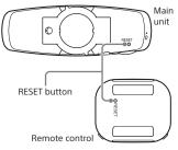
If the problem persists even after the resetting operation above, initialize the main unit as follows Press and hold the RESET button for about 15 seconds with something fine-tipped such as a hairpin. The indicator (blue) flashes 4 times, and the main unit is reset to the factory settings. All pairing information is deleted.
