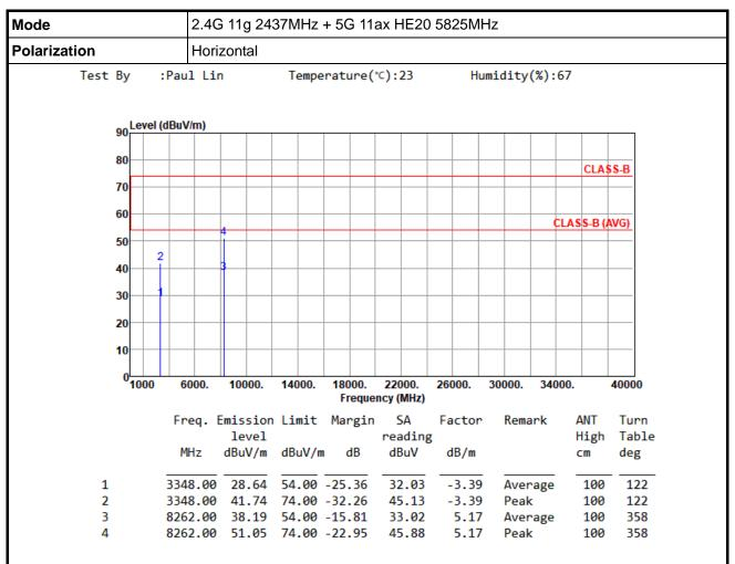
Note 1: Emission Level (dBuV/m) = SA Reading (dBuV/m) + Factor\* (dB/m)
