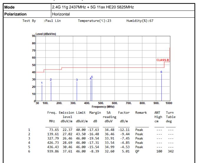
Note 1: Emission Level (dBuV/m) = SA Reading (dBuV/m) + Factor\* (dB/m)
