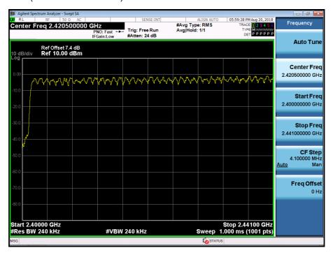
Test Plots (π/4DQPSK) Number of Channels (2.441 GHz - 2.4835 GHz)
