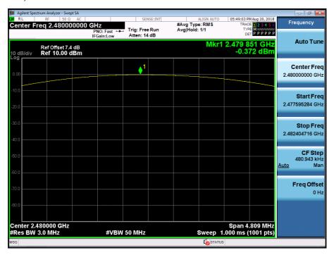
Test Plots (8DPSK) Peak Power (CH.0)
