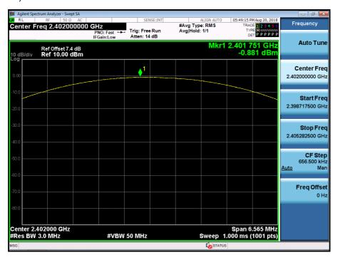
Test Plots (π/4DQPSK) Peak Power (CH.39)
