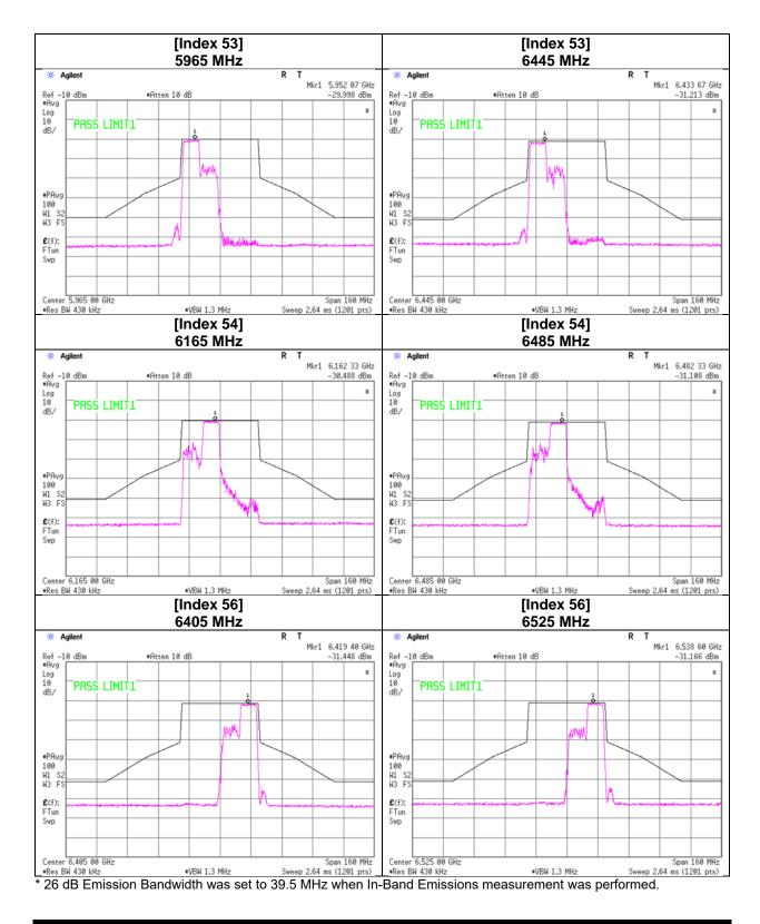
Test place Date Temperature / Humidity Engineer Mode Ise EMC Lab. No.8 Measurement Room February 1, 2024 22 deg. C / 39 % RH Takumi Nishida Tx 11be-40 [106-tone RU]
