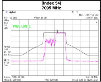
\* 26 dB Emission Bandwidth was set to 19.8 MHz when In-Band Emissions measurement was performed.
