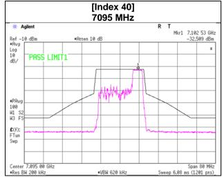
\* 26 dB Emission Bandwidth was set to 19.8 MHz when In-Band Emissions measurement was performed.
