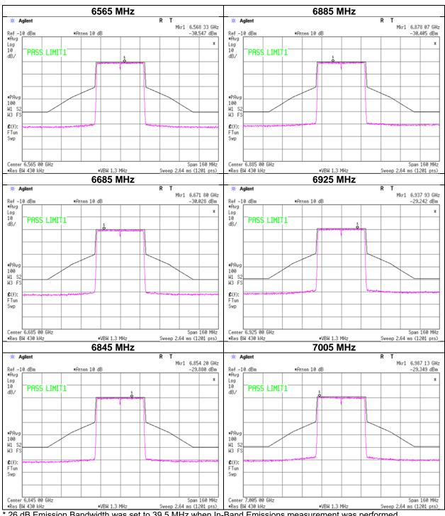
26 dB Emission Bandwidth was set to 39.5 MHz when In-Band Emissions measurement was performed.
