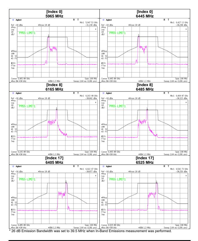
Test place Date Temperature / Humidity Engineer Mode Ise EMC Lab. No.8 Measurement Room January 30, 2024 22 deg. C / 40 % RH Takafumi Noguchi Tx 11be-40 [26-tone RU]
