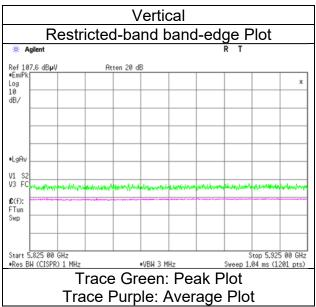
\* The measurement was conducted for a sufficiently long enough time to detect any possible spurious emissions.
