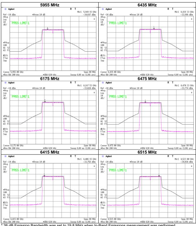
26 dB Emission Bandwidth was set to 19.8 MHz when In-Band Emissions measurement was performed.
