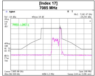
\* 26 dB Emission Bandwidth was set to 39.5 MHz when In-Band Emissions measurement was performed.
