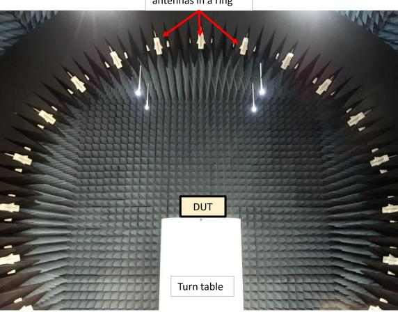
Dual-polarized antennas in a ring
