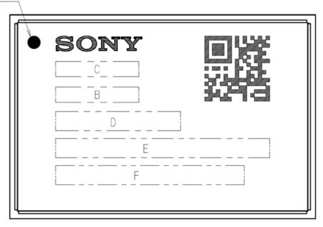
MARKING C: M1502 D: E: FCC ID: AK8M1502 F: IC: 409B-M1502
