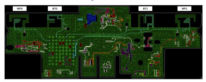
Please use supplied Gerber file and PCB material info for antenna connection trace design.
