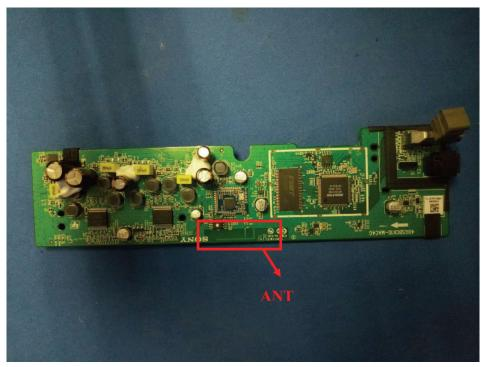
**Figure 22** Inside of the EUT
