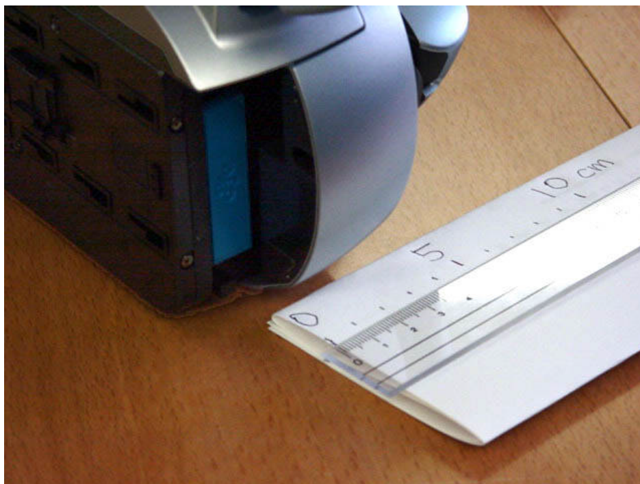
These photos show how Wireless LAN card is installed in the toy. Blue part in the body of toy is an antenna of the wireless LAC card "ERA-201D1".
