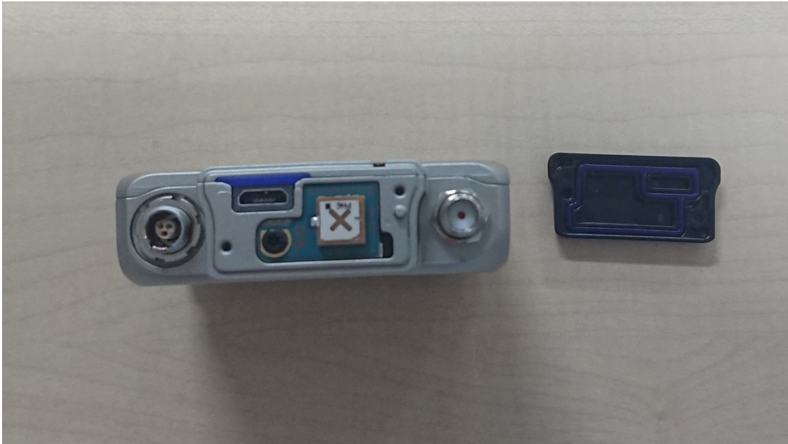
Fig1: Removed the antenna cover
