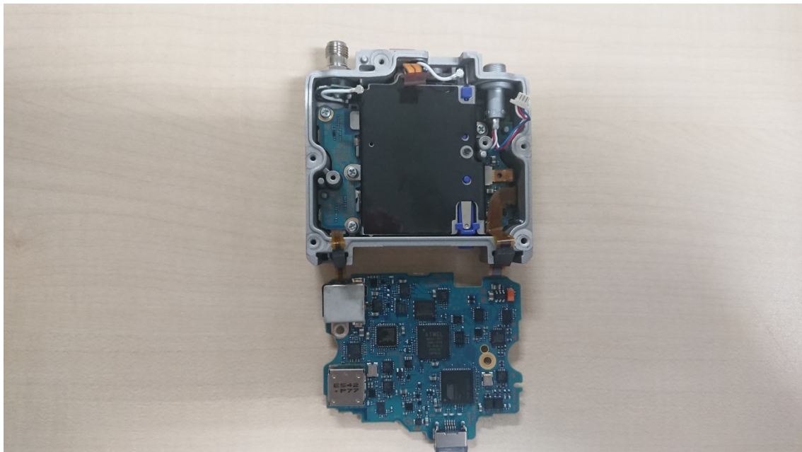
Fig4: Removed the board TX-162, main block
