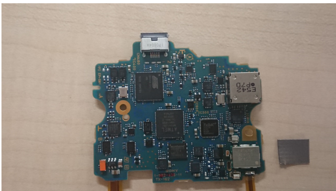
Fig.12: Removed the electromagnetic absorber sheet
