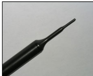
EX3DV4 E-field Probe
