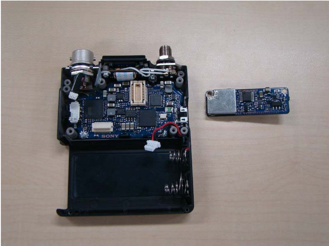
Fig.5: Removed the board TX-147
