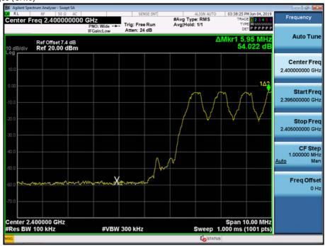
Test Plots with hopping (GFSK)
