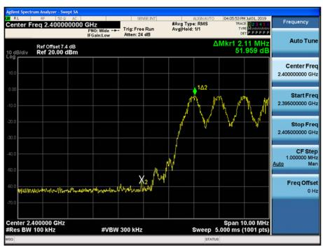
Test Plots with hopping (GFSK)
