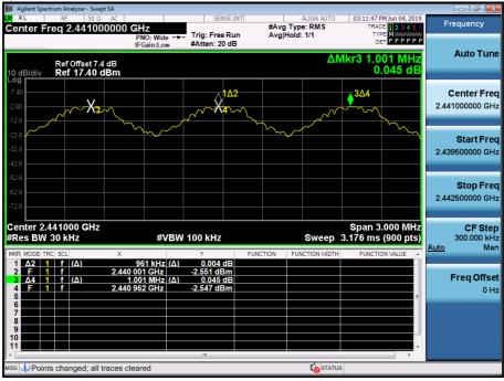
Test Plots (8DPSK) Channel Separation
