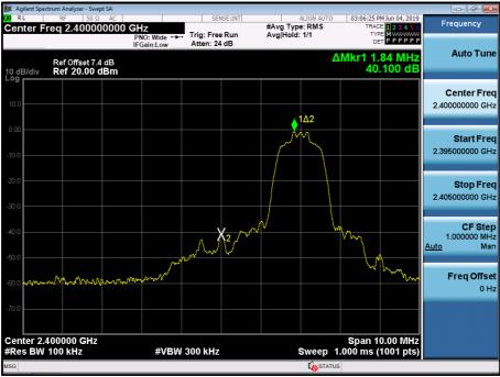
Test Plots without hopping (π/4DQPSK) Band Edges (CH.78)
