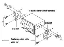
When mounting this unit to the preinstalled brackets of your car, use the mounting screws (1) in the appropriate screw holes based on your car: T for TOYOTA and N for NISSAN.
