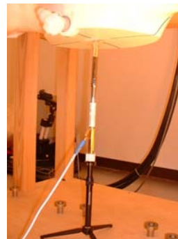
2450MHz System performance check setup
