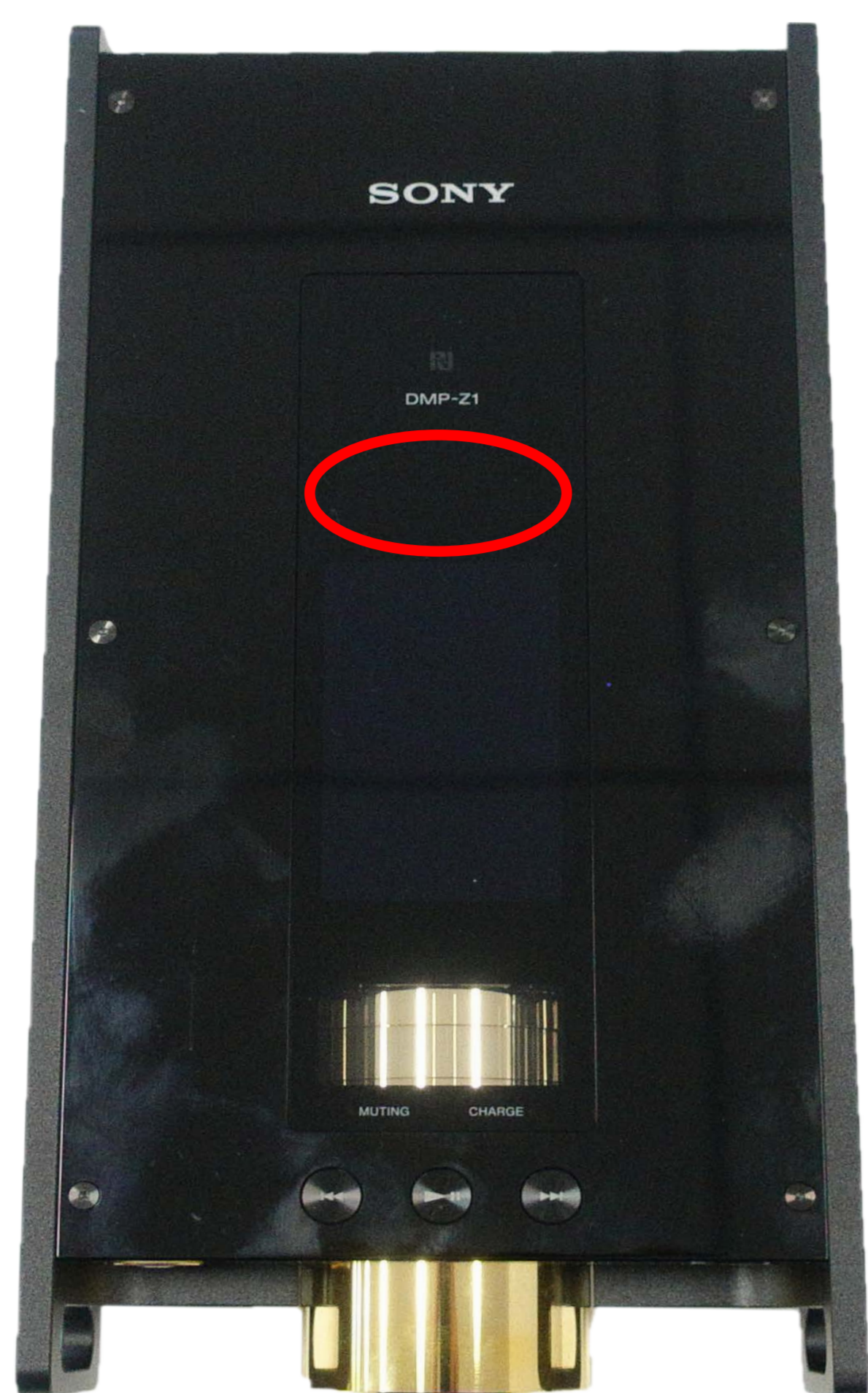
DMP-Z1 Bluetooth Antenna Position
