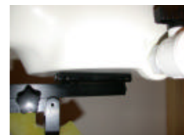
Figure 13.1 Body SAR Test Setup -- Front Side Position --
