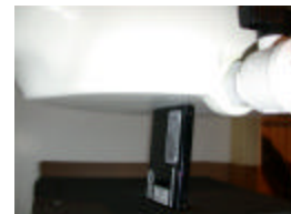
Figure 13.3 Body SAR Test Setup -- Top Side Position --
