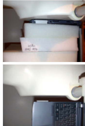
Figure 8.1 Body SAR Laptop and Bystander Configurations
