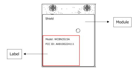
FCC ID is described on top of Module. Labeling meets the conditions allowed in KDB784748. FCC part15 statement in manual, when it would be embeded on Host.
